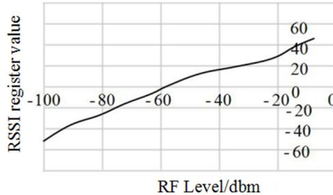
Fig. 2. Relation between RSSI value and input power
