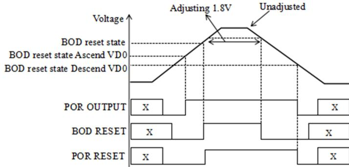
Fig. 4. Relations between power-on reset and brown-out detection
